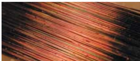
PHOTONIC-CRYSTAL THREADS are 0.2 millimeter wide.
